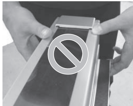
Do not transport the actuator by holding its guide rail.
