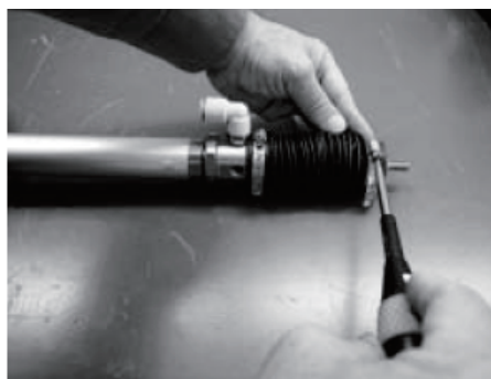
Loosening of front metal fitting
