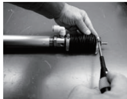
Tightening of front metal fitting
