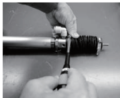
Loosening of rear metal fitting
