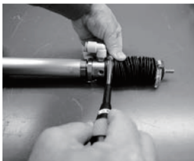
Tightening of rear metal fitting
