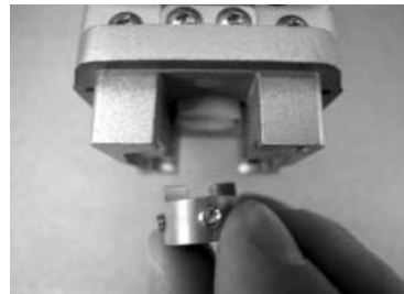
Inserting the coupling (with screws)
