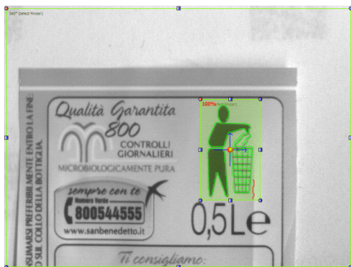
Fig. A 360° Defect Finder Control: Reference Image
